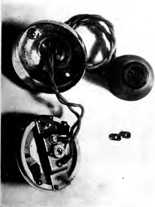
FIG. 22.—AMERICAN TRANSMITTER WITH COVER REMOVED.
